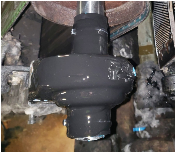
Above: Enviropeel-protected bearings at a drywall production facility
