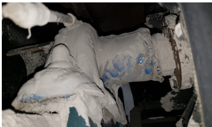
Enviropeel is seen above being applied at an asphalt shingle plant. This was a second visit to the plant following an 800% improvement in bearing life in areas where Enviropeel had previously been applied. Left: After a year at a drywall plant, an Enviropeel protected bearing is buried in gypsum dust. Note the accumulation around the end of the shaft - nothing is getting into the bearing through here!
