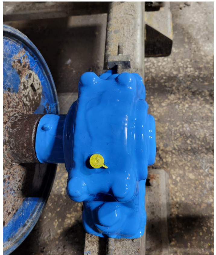
Enviropeel is seen above being applied at an asphalt shingle plant. This was a second visit to the plant following an 800% improvement in bearing life in areas where Enviropeel had previously been applied. Left: After a year at a drywall plant, an Enviropeel protected bearing is buried in gypsum dust. Note the accumulation around the end of the shaft - nothing is getting into the bearing through here!
