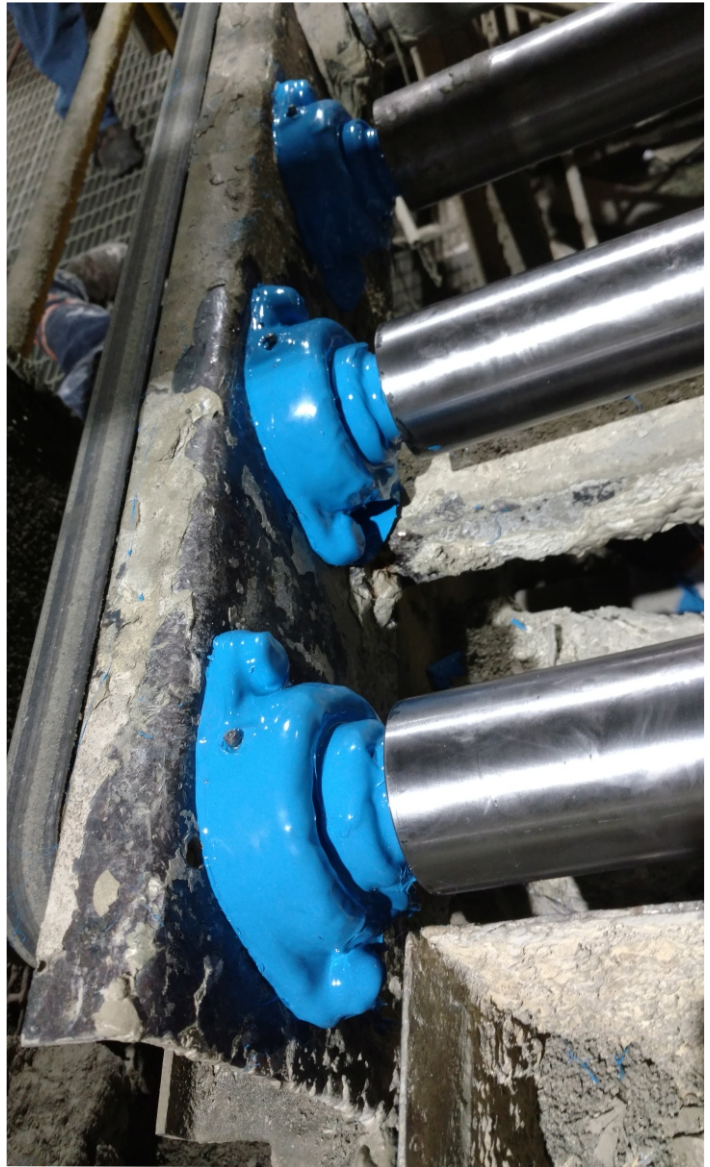
Above: Enviropeel-protected bearings at a drywall production facility
