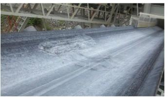
The photos of the repaired belt, shown left, were taken eighteen months after the repair was completed.
