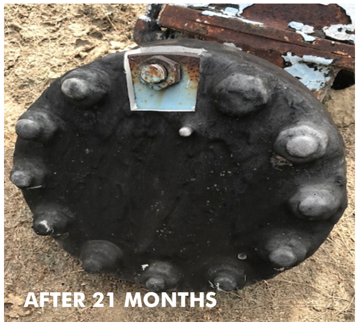
Below right: inspection reveals substrate to be in original condition without any further corrosion despite flooding.
