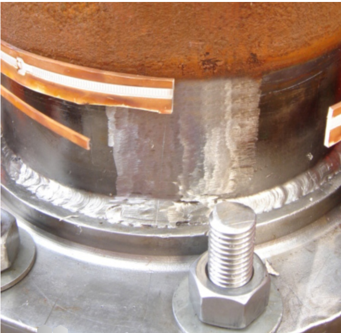
Figure.11 below: cutting through the sealing tie reveals a sharp line between the protected and unprotected areas of
