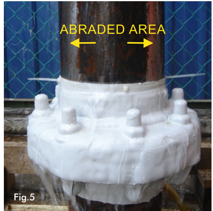
Fig.5 above: substrate and Enviropeel encapsulation shortly after the beginning of the trial. On potentially vulnerable edges, cable ties provide extra security.
