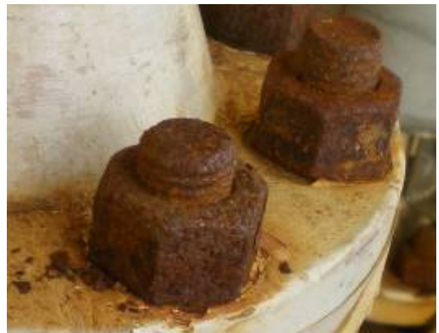
Figures 4 and 5: zinc-nickel plated L7 bolts on a mixed stainless/carbon steel substrate
