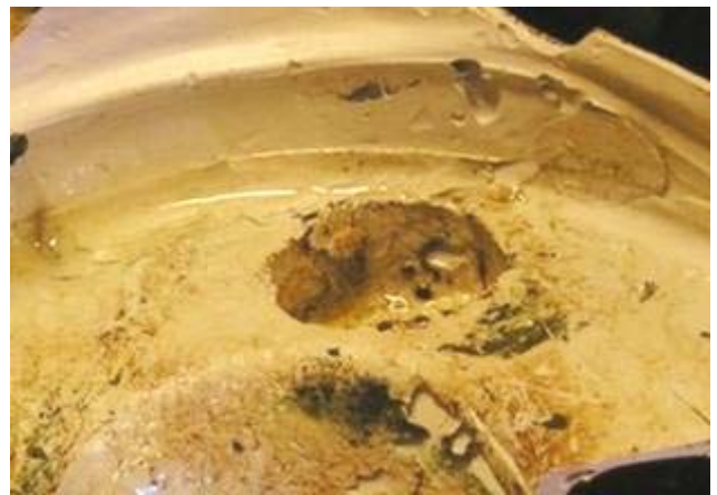
Figures 10 and 11: sample removal shows previously rusting substrate and inner surface of CIST encapsulation coated with oil
