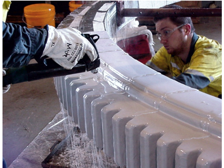
Top: A large steel mining component is being prepared for long-term storage using Enviropeel
